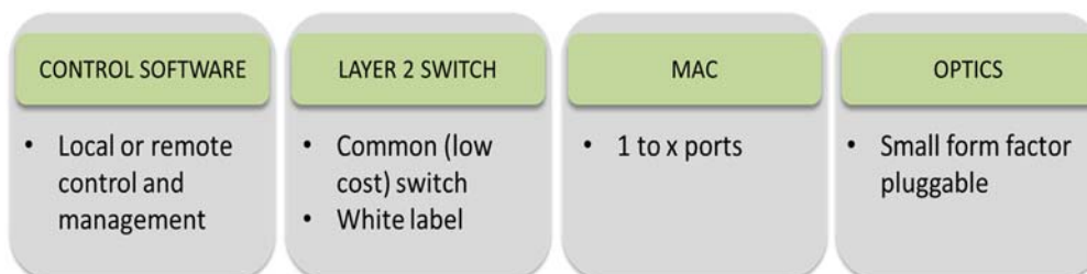
Figure 9: Modularized Functions of the OLT
